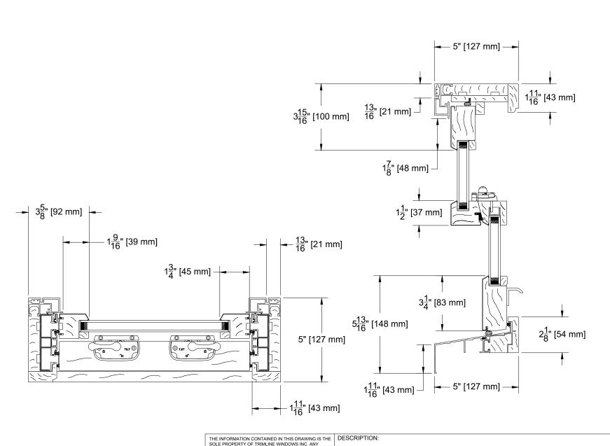
ECLIPSE | LEGENDS SERIES ALUMINUM CLAD-WOOD DOUBLE HUNG FULL JAMB THE INFORMATION CONTAINED IN THIS DRAWING IS THE SOLE PROPERTY OF TRIMLINE WINDOWS INC. ANY REPRODUCTION IN PART OR AS A WHOLE WITHOUT THE WRITTEN PERMISSION OF TRIMLINE WINDOWS INC. IS PROHIBITED.
