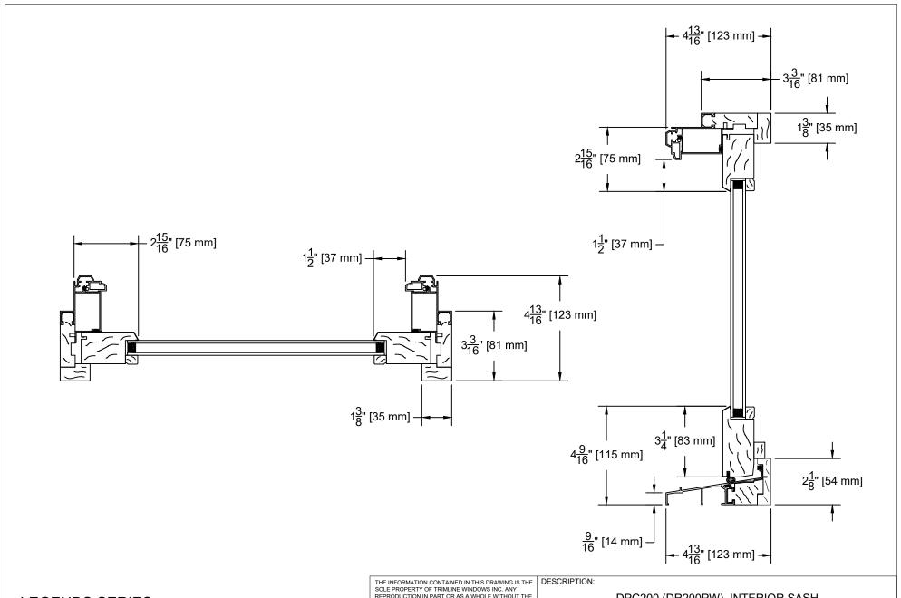
**LEGENDS SERIES ALUMINUM CLAD-WOOD DOUBLE HUNG PICTURE** POCKET INSERT REPLACEMENT FRAME
