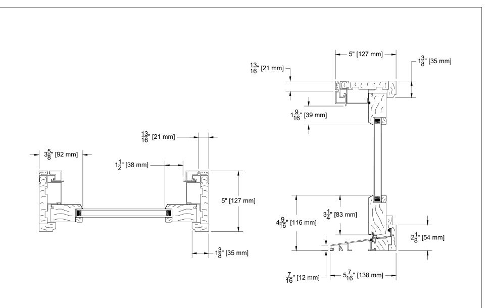
ECLIPSE | LEGENDS SERIES ALUMINUM CLAD-WOOD DOUBLE HUNG PICTURE FULL JAMB THE INFORMATION CONTAINED IN THIS DRAWING IS THE SOLE PROPERTY OF TRIMLINE WINDOWS INC. ANY REPRODUCTION IN PART OR AS A WHOLE WITHOUT THE WRITTEN PERMISSION OF TRIMLINE WINDOWS INC. IS PROHIBITED.
